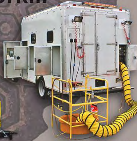
Truck Genset Delivery System Manhole Support
